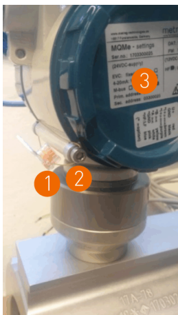
Fig. 8: Seal and safety screw
